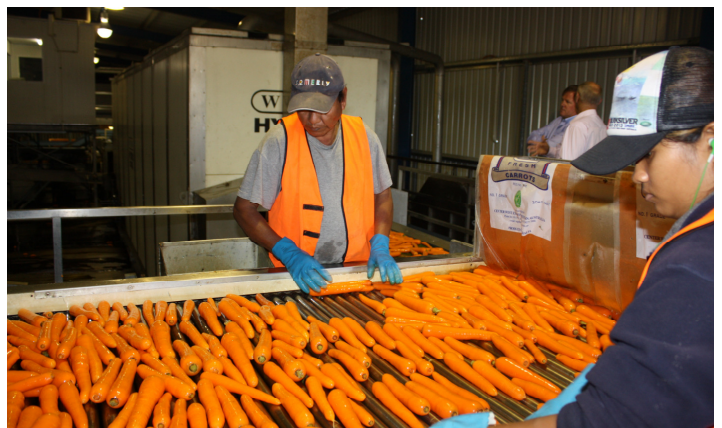
Carrots are washed and graded before being processed through the hydrocooler where they are chilled to the core
